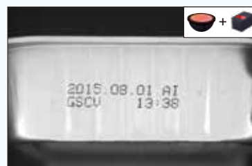
Allows for uniform imaging of the whole container by combining the Dome Light with a Coaxial Light.
