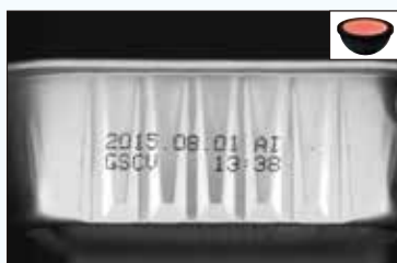
Imaging with Dome Light captures reflections from the bumps on the container.
