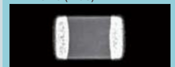
Condensed illumination (condensed by three independent arrays) with wide field of view
