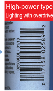
Shutter speed: 1/18,000 Lighting with overdrive: 100% intensity
