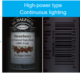
Shutter speed: 1/10,000 Amount of light: 100% intensity Continuous lighting: 100% intensity
