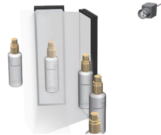
Inspection with a line sensor camera
