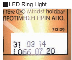
Converged light in the center interferes with stable inspection.
