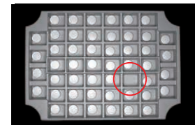
The whole thing is illuminated evenly, allowing for detection of present contents.
