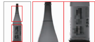
The liquid surface level and the label position are clearly imaged.
