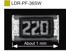
The appearance of the chip component is captured.
