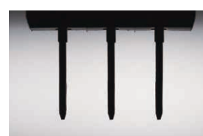
Illumination using a diffusion plate from behind the workpiece allows you to observe the appearance of the connector.
