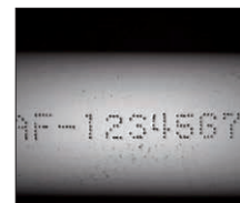
Inspecting dot-marked characters on pipe Light used: LSP-41RD
