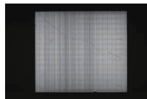
Due to reflection from the hairline finishing surface, it is difficult to form an image of the damage.
